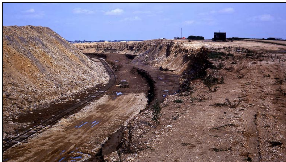
Figure 6. Colsterworth Pit No.2 in 1966, looking east, with Northampton Sand Formation overlain successively by the Grantham Formation and the Lincolnshire Limestone; compare this photograph with Plate 1A in Hollingworth and Taylor, 1951.
